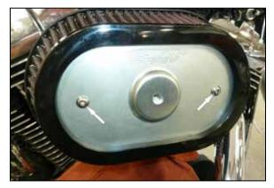
10. Place the K&N<sup>®</sup> filter on the back plate and attach with the remaining button head screws. **NOTE: Apply one drop of provided thread locker to each screw.**
