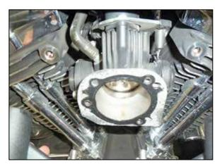
6. Remove the backing plate and stock gasket. NOTE: K&N Engineering, Inc. recommends that
