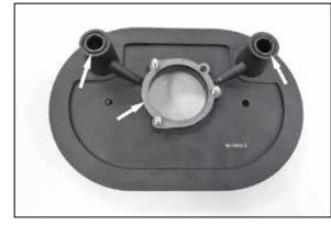
8. Install the remaining two O rings and the two filter spacers onto the front of the K&N<sup>®</sup> back plate as shown using the provided hardware.
