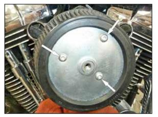
3. Remove the remove the three Torx screws that attach the air filter.
