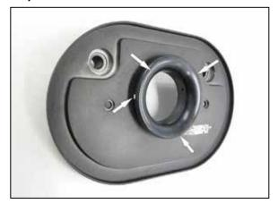
7. Install the provided intake velocity stack and the three throttle body bolts in the  $K\&N^{\otimes}$  back plate.
